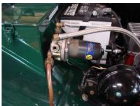
Disconnected the fuel lines, the 2 power wires, and unbolted it from the tool box. Darn Whitworth bolts.
