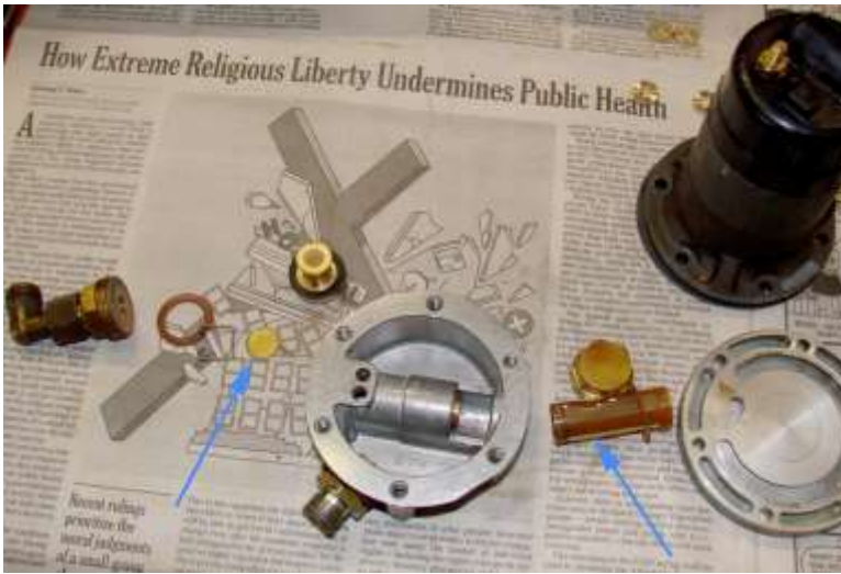
The lower assembly with the old strainer to the right of the lower aluminum housing, & one of the brass check valve discs to the left. Fuel flows in lower left, thru strainer, out left.
