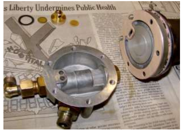
All ready to screw back together. Bottom of the diaphragm spacer & gaskets on right. Old check valve parts above.
