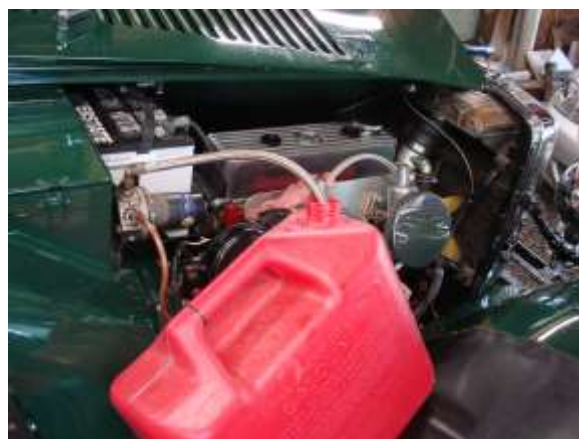
Testing the pump: pumping fuel into a gas can, engine not running. No failure – it worked perfectly for several gallons.
