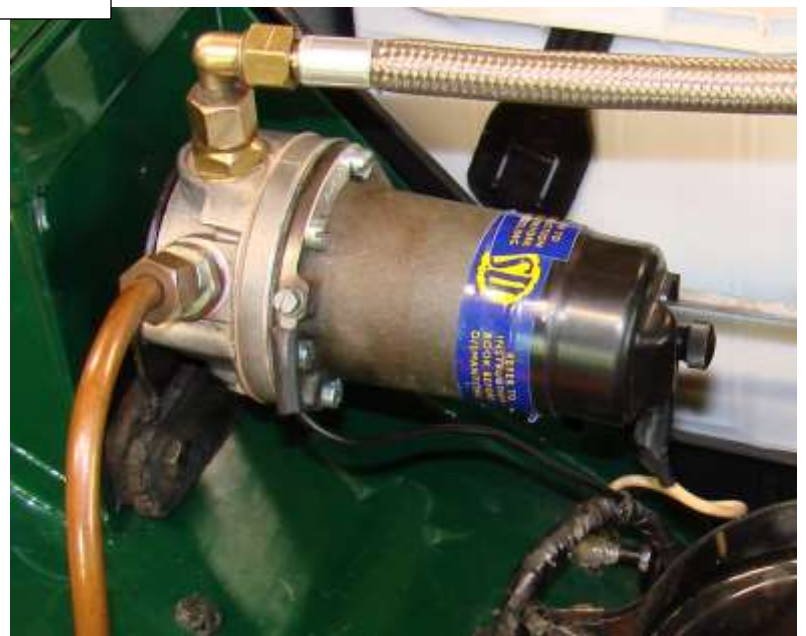
Pump is screwed onto its bracket, bracket bolted back onto the tool box. Wires & fuel lines all hooked up.
