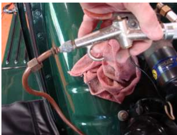
I blew out the fuel line to make sure it wasn't plugged at the tank outlet
