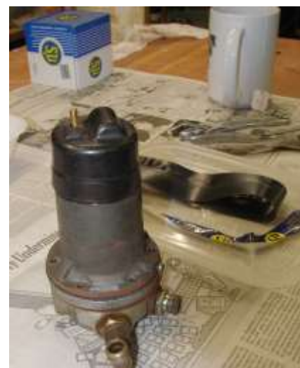
The tape covers the joint between the plastic cap and the iron solenoid housing
