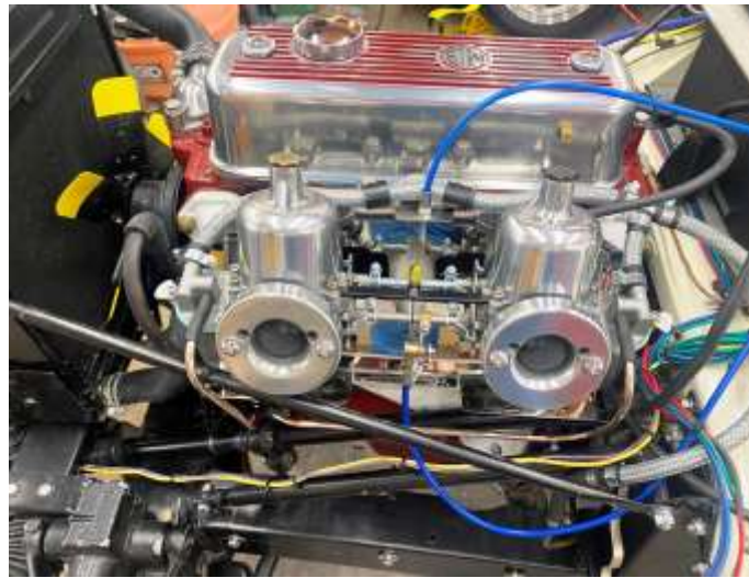
“..the intake horns were polished, mesh intake screens made, the decision was made to run without filters.”
