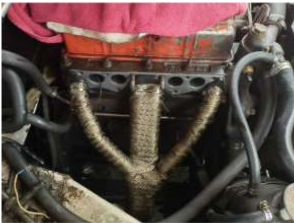
The finished, installed exhaust manifold. "...I really just like wrapped headers..."
